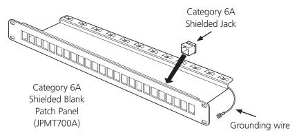
Figure 2. Installing the jacks into the patch panel.
